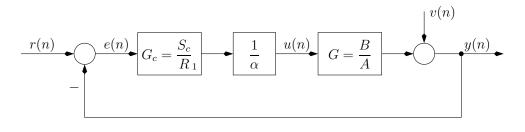
$$Y(z^{-1}) = \frac{\frac{S}{R_1} \frac{1}{\alpha} \frac{B}{A}}{1 + \frac{S}{R_1} \frac{1}{\alpha} \frac{B}{A}} R + \frac{1}{1 + \frac{S}{R_1} \frac{1}{\alpha} \frac{B}{A}} V$$
