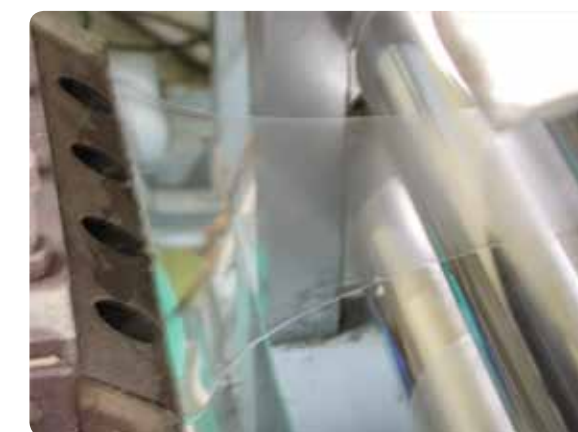
Molten PVDF polymer being extruded as a film onto a cast roll. (Mhalgi, Khakhar and Misra, Polym. Eng. Sci. , 2007)
