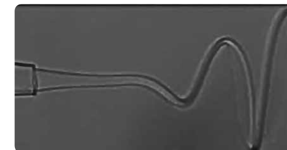
Controlled whipping of an electrified jet in the presence of a coflowing external liquid
