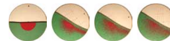
Mixing of particles in a rotating cylinder. (Hajra and Khakhar, Phys. Fluids , 2005)
